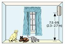
Mount the detector 7.5 to 9 feet (2.3 to 2.7 meters) above the floor
